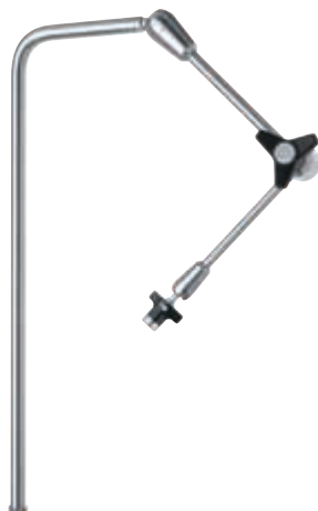
28272 HB Articulated Stand , reinforced version, L-shaped, with one central clamp for all five joint functions, height 48 cm, operating range 52 cm, with quick release coupling KSLOCK (female)
